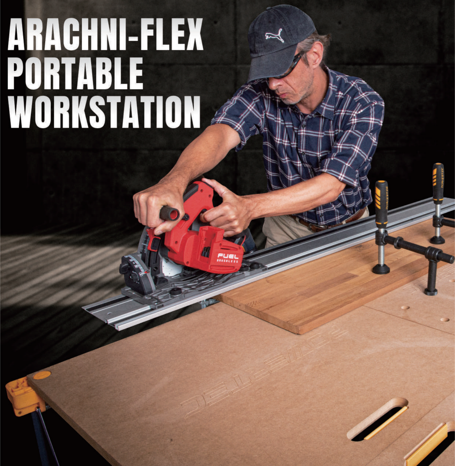
71928 2ft x 8ft, 36" Work Height 2,500 lbs Loading Capacity
