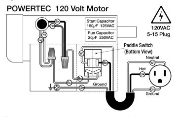
The permanently split capacitor motor has the following specifications:
