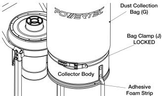
15. Secure in place with the second Quick Release Bag Clamp.
