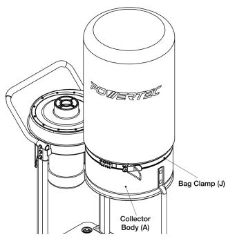
13. See Figure 10. Remove the backing from the Adhesive Foam Strip (supplied) and place it onto the bottom grooved rim on lower opening of the Collector Body.
