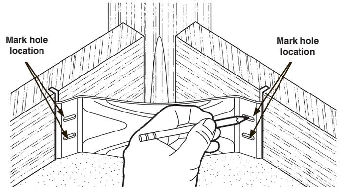
8. Secure the corner brackets to the apron pieces with the #10 x 5/8" pan head screws.
