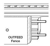
Square jointing rods shown in the square grooves for the 5/64" offset.
