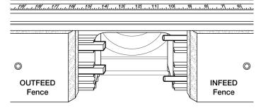
Square jointing rods shown in the square grooves on the OUTFEED fence. Round jointing rods in the round grooves on the INFEED fence for the **3/128" offset.**
