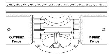
Install a straight bit in the router. Place a straight edge against the outfeed fence face and position the fence so the bit just grazes the straight edge.
