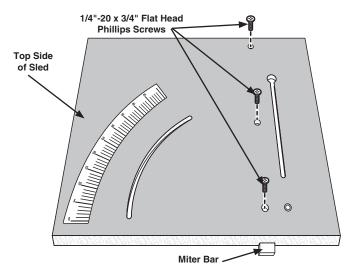
From the underside of the sled, insert the two 1/4"-20 x 3/4" flat head Phillips screws through th pre-drilled holes and attach the adjustable stop to the table. Make sure the set screw is positioned to the outer edge of the sled and the side marked with a "O" is facing up. See Figure 4.
