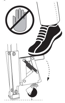
To retract, step on lower lever and the caster assembly will "snap" up, lowering the leg.
